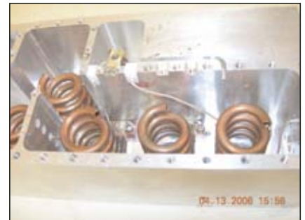
▲ Fig. 5 Capacitive cross-coupling.
