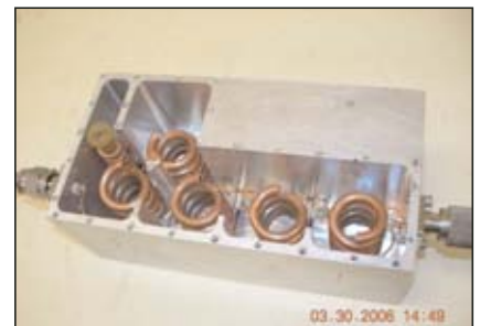
▲ Fig. 6 Helical resonator filter with capacitive (through-the-opening) cross-coupling and a trap resonator.
