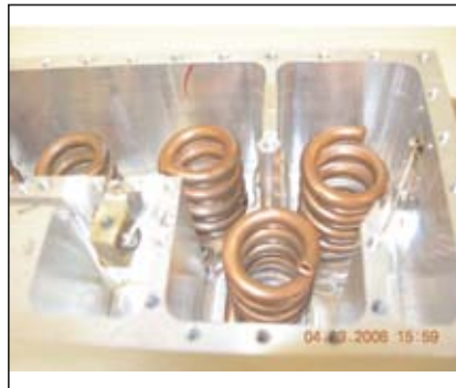
Fig. 12 Filter with 3rd and 5th resonators inductively coupled with wire and capacitively coupled resonators 1 and 3.
